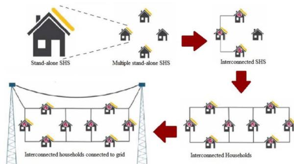
Figure 2: Swarm Electrification concept and stepwise approaches [66]
